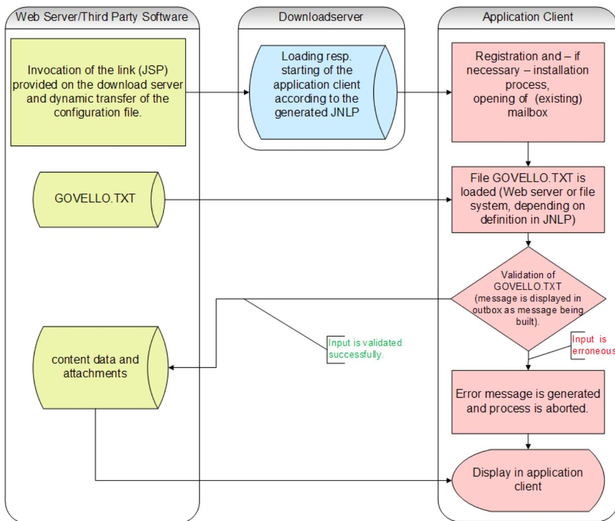
Figure 3: Outline and flowchart of the dynamic data transfer interface
